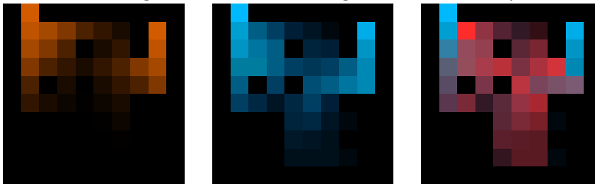
Images (left to right): slice of the light voxel map using LPV, slice of the light voxel map using SGI, difference between the two where red is a larger difference. Notice that using LPV, light does not converge throughout the entire scene and does not cast secondary shadows.
